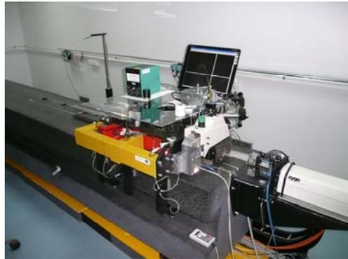
Fig. 1 Experimental setup of the length comparator and the microscope
